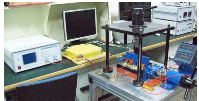
Fig. 2 Measuring device for magnetic properties allowing for stress dependency
