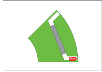
Fig. 4. Maximum stress position (Initial design plan)
